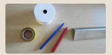
Stick a paper strip on the rope, draw a straight line on it and pass a chalk stick to reveal the track. Then make the measurement directly on the paper strip.
